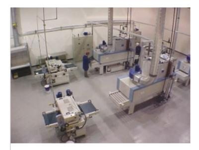
Opened in 2001, the Arch Coatings R&D operation in Brandenburg, Ky., represents a \$1 million investment. Equipped with advanced application and drying systems, the center has a low-pressure UV curing unit for fully pigmented UV coatings and can reproduce numerous combinations of air, infrared, and UV drying. An even larger research facility exists at the head-quarters of Arch Coatings in Italy.
